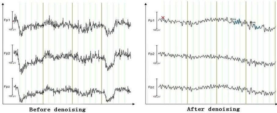
Figure 4. Comparison of before and after denoising of EEG signals collected by experiment
